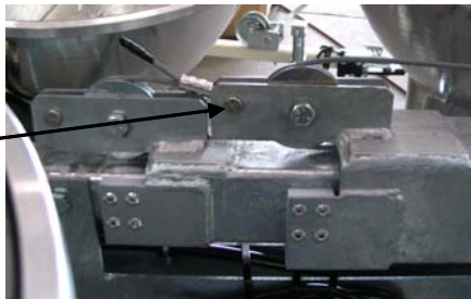
Figure 2. Cable Routed Through Pulley
