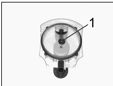
Skruva loss flottören (1)
